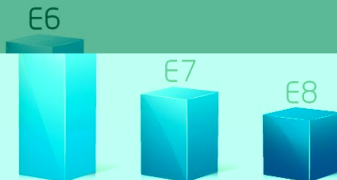
COMPARISON IN WEIGHT LOSS IN 10% H 2 SO 4 SOLUTION AT 96°C FOR 24 HOURS
